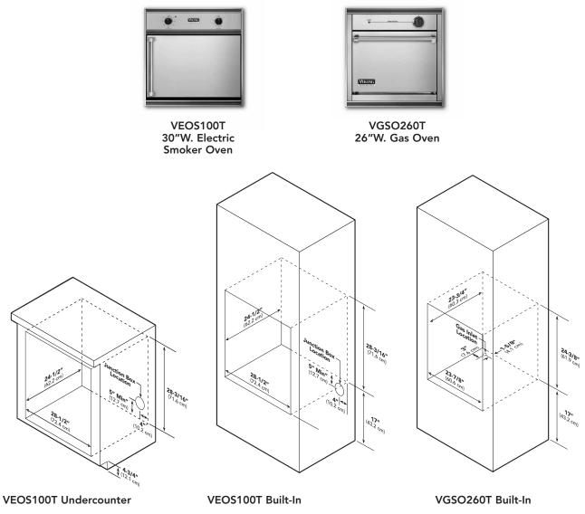
**Note:** The use of cabinets for storage above the oven may result in a potential burn hazard. Combustible items may ignite, and metallic items may become hot and cause burns. If cabinet storage is to be provided, the risk can be reduced by installing a hood that projects horizontally a minimum of 5" (12.7 cm) beyond the bottom of the cabinets. Do not obstruct the flow of combustion and ventilation air.
